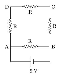
A 16  $\Omega$  resistance wire is bent to form a square. A source of emf 9 V is connected across one of its sides as shown. Calculate the current drawn from the source. Find the potential difference between the ends C and D.
