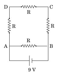
A 16  $\Omega$  resistance wire is bent to form a square. A source of emf 9 V is connected across one of its sides as shown. Calculate the current drawn from the source. Find the potential difference between the ends C and D.
