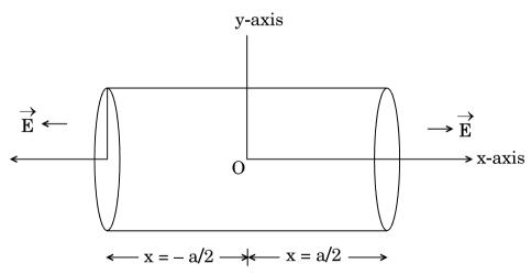
Find out the flux (i) through the flat faces, (ii) through the curved surface of the cylinder. What is the net outward flux through the cylinder and the net charge inside the cylinder?
