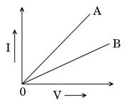
I-V graph for two identical conductors of different materials A and B is shown in the figure. Which one of the two has higher resistivity?
