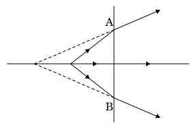
The line AB in the ray diagram represents a lens. State whether the lens is convex or concave.
