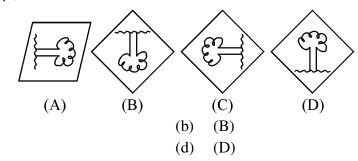
A student is performing the experiment of determining the focal length of a given concave mirror by focusing a distant tree on a screen. Which one of the following kinds of images he is likely to obtain on the screen?
