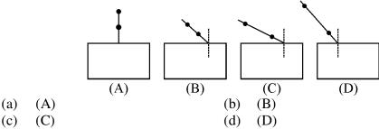
Study the following four experimental setups by four students A, B, C and D showing the incident ray to trace the path of a ray of light through a glass slab. Which of these will get the best result?
