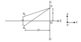
At centre of the screen i.e. at point O, waves from two sources  $S_1$  and  $S_2$  meet in same phase and produce constructive interference, and similarly at all those points on the screen where waves have path difference  $n_{\lambda}$ , n=0,1,2,3 ..., they produce constructive interference hence bright fringes are obtained.
