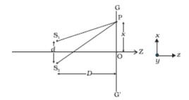
At centre of the screen i.e. at point O, waves from two sources  $S_1$  and  $S_2$  meet in same phase and produce constructive interference, and similarly at all those points 1
