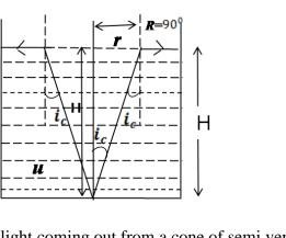
It is only the light coming out from a cone of semi vertical angle  $i_c$  ( $i_c = \sin^{-1}\frac{1}{\mu}$  = critical angle) that needs to be stopped by the opaque disc
