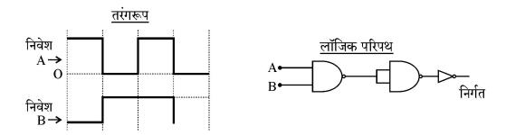
Using the input A and B, waveforms, draw the output waveform of the given logic circuit. Identify the logic gate obtained. Write its truth table.
