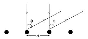
Two reflected waves will interfere. The interference is due to de Broglie wave of the electron accelerated from rest by less then  $1~{\rm keV}.$
