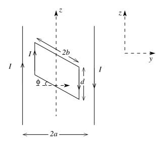
(a) Obtain the torque tending to rotate the rectangular loop about its axis as a function of  $\phi$ . Here  $\phi$  is the angle that plane of loop makes with the plane of wires.
