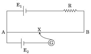
In the circuit diagram shown, AB is a uniform wire of resistance 15  $\Omega$  and length 1 m. It is connected to a cell  $E_1$  of emf 2 V and negligible internal resistance and a resistance R. The balance point with another cell  $E_2$  of emf 75 mV is found at 30 cm from end A. Calculate the value of the resistance R.
