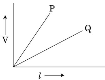
The variation of potential difference  $V$  with length  $l$  in case of two potentiometers wires P and Q is as shown. Which one of these will you prefer for comparing emfs of two primary cells and why ?
