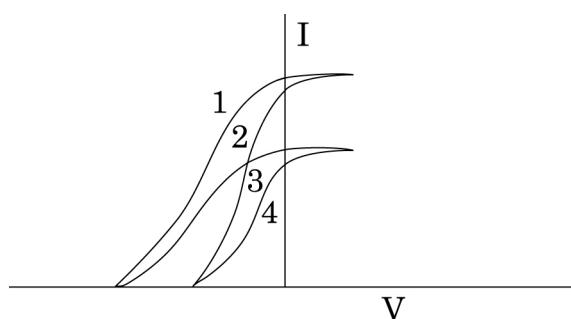
The given graph shows the variation of photo-electric current(I) with the applied voltage(V) for two different materials and for two different intensities of the incident radiations. Identify and explain using Einstein's photo electric equation the pair of curves that correspond to (i) different materials but same intensity of incident radiation, (ii) different intensities but same materials.
