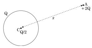
A thin metallic spherical shell of radius R carries a charge Q on its surface. A point charge Q/2 is placed at the centre C and another charge +2Q is placed outside the shell at A at a distance x from the centre as shown in the figure.
