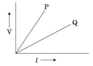
The variation of potential difference V with length l in case of two potentiometers wires P and Q is as shown. Which one of these will you prefer for comparing emfs of two primary cells and why?
