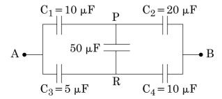
Calculate the equivalent capacitance between points A and B in the circuit below. If a battery of 10 V is connected across A and B, calculate the charge drawn from the battery by the circuit.
