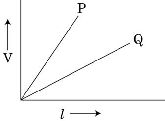
The variation of potential difference  $V$  with length  $l$  in case of two potentiometer wires P and Q is as shown. Which one of these will you prefer for comparing emfs of two primary cells and why?
