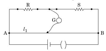
An unknown resistance X is now connected in parallel to the resistance S and the balance point is found at a distance  $l_2$ . Obtain a formula for X in terms of  $l_1$ ,  $l_2$  and S.
