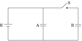
Two identical parallel plate capacitors A and B are connected to a battery of V volts with the switch S closed. The switch is now opened and the free space between the plates of the capacitors is filled with a dielectric of dielectric constant K. Find the ratio of the total electrostatic energy stored in both capacitors before and after the introduction of the dielectric.
