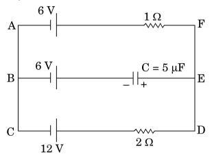
In the given circuit, with steady current, calculate the potential difference across the capacitor and the charge stored in it.
