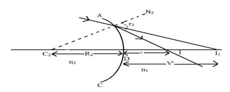
Suppose we have a thin lens of material of refractive index n2, placed in a medium of refractive index  $n_1$ , let  $0 \text{ be } a_n$ .
