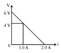
The figure shows a plot of terminal voltage 'V' versus the current 'i' of a given cell. Calculate from the graph (a) emf of the cell and (b) internal resistance of the cell.
