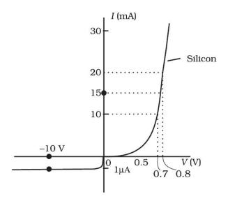
The V-I characteristic of a diode is shown in the figure. The ratio of the resistance of the diode at I = 15 mA to the resistance at V = -10 V is
